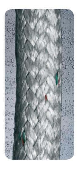
CHEMICAL RESISTANCE - good SPECIFIC GRAVITY - 1,38 MELTING POINT - approx 260° C
